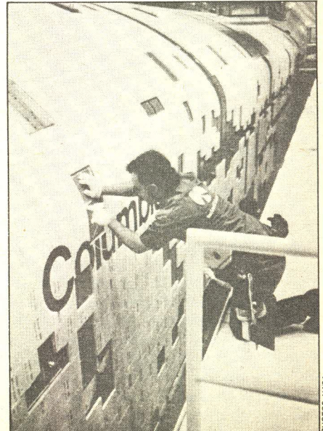
Tile replacement and repair continues.
